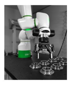
"MOVES SIMILARLY TO THE HUMAN ARM WITH SEVEN JOINTS, ONE METER REACH, AND THE ABILITY TO LIFT 5KG OR 11LBS. 0B7 IS ABLE TO MANEUVER INTO TIGHT SPACES AND CAN EASILY ADAPT TO YOUR EXISTING MANUFACTURING ENVIRONMENT."
